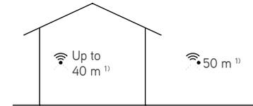
Casambi uses mesh network technology so each output module acts also as a repeater. Longer ranges can be achieved by using multiple casambi ready output units.
