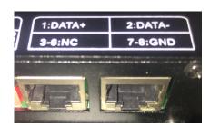
DMX signal port interface, two network port terminals are connected in parallel, port 1 is DATA+, port 2 is DATA-, port 3-6 is empty, port 7, 8 is GND.
