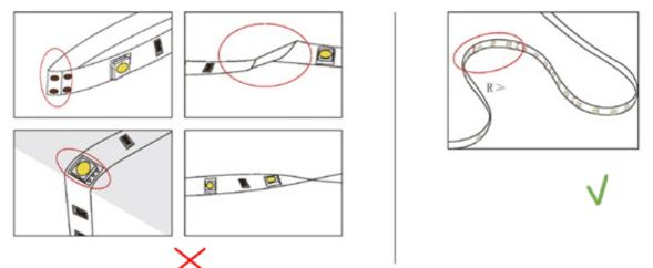
minimum bending radius is given in the datasheet coupled to the article number on the website.
